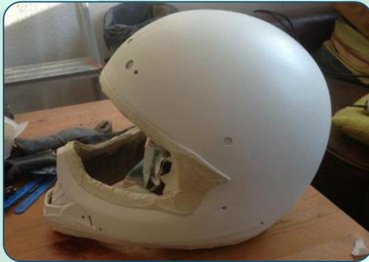
I had to apply several layers until an optimal coverage appeared. After that, the coating layer had to be grinded and degreased again. As the glue of the masking tapes could react with the components of the varnish and could leave residues on the surface, I had to wait a few days until the subsurface was ready for further handling.
